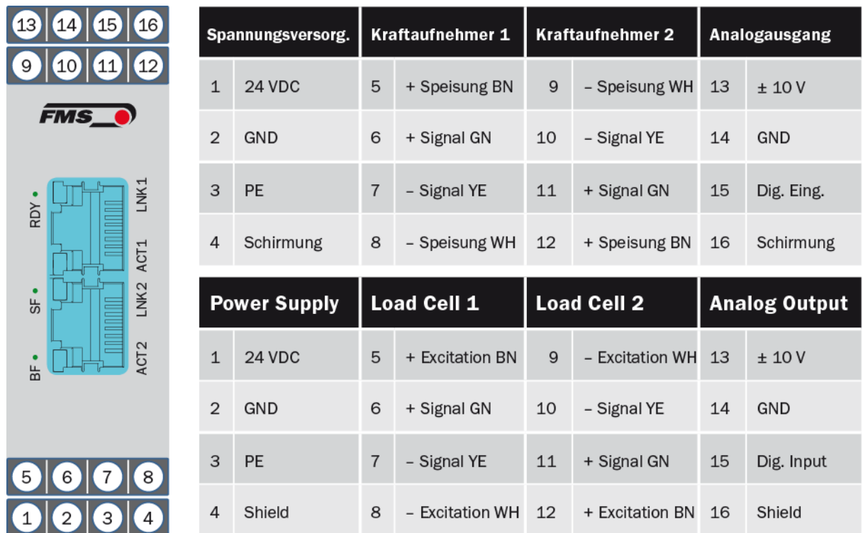
Fig. 2a: Wiring Diagram EMGZ490A.R
