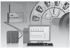
**RTM** (Radio Transmitted Tension Monitoring) delivers system solutions across the cable production value chain. These innovative systems utilise force measuring rollers to capture the tension of individual wires or strands, and then securely transmit this data from the rotating to the static part of the machine. The systems are designed with fully compatible components. Production rates and product quality on rotating strand-handling machinery are significantly improved.
