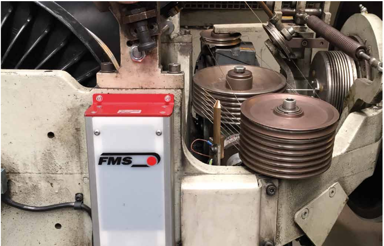
RTM MP | Typical Application in Bow Type Stranding Machine
