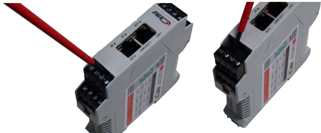
Figure 3: Detachable terminal blocks: use a small slotted screwdriver as a lever
