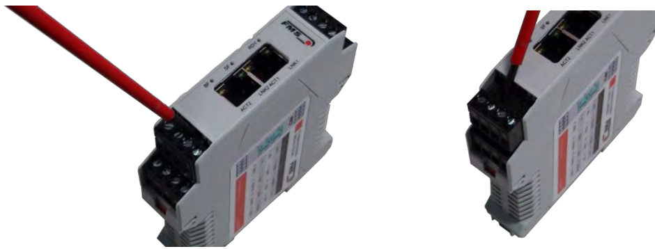
Figure 3: Detachable terminal blocks: use a small slotted screwdriver as a lever
