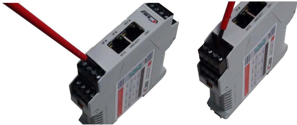
Figure 3: Detachable terminal blocks: use a small slotted screwdriver as a lever
