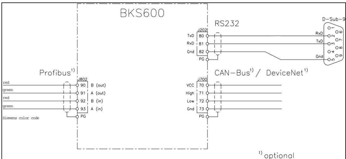
fig. 12: Wiring of the interfaces
