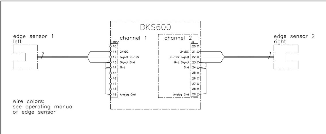
fig. 9: Wiring of the edge sensors
