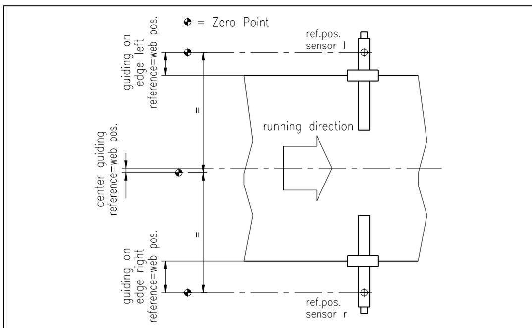
**fig. 19: Calculation of the reference value during automatic start by using linear units (without reference point on the machine frame)** K601009e
