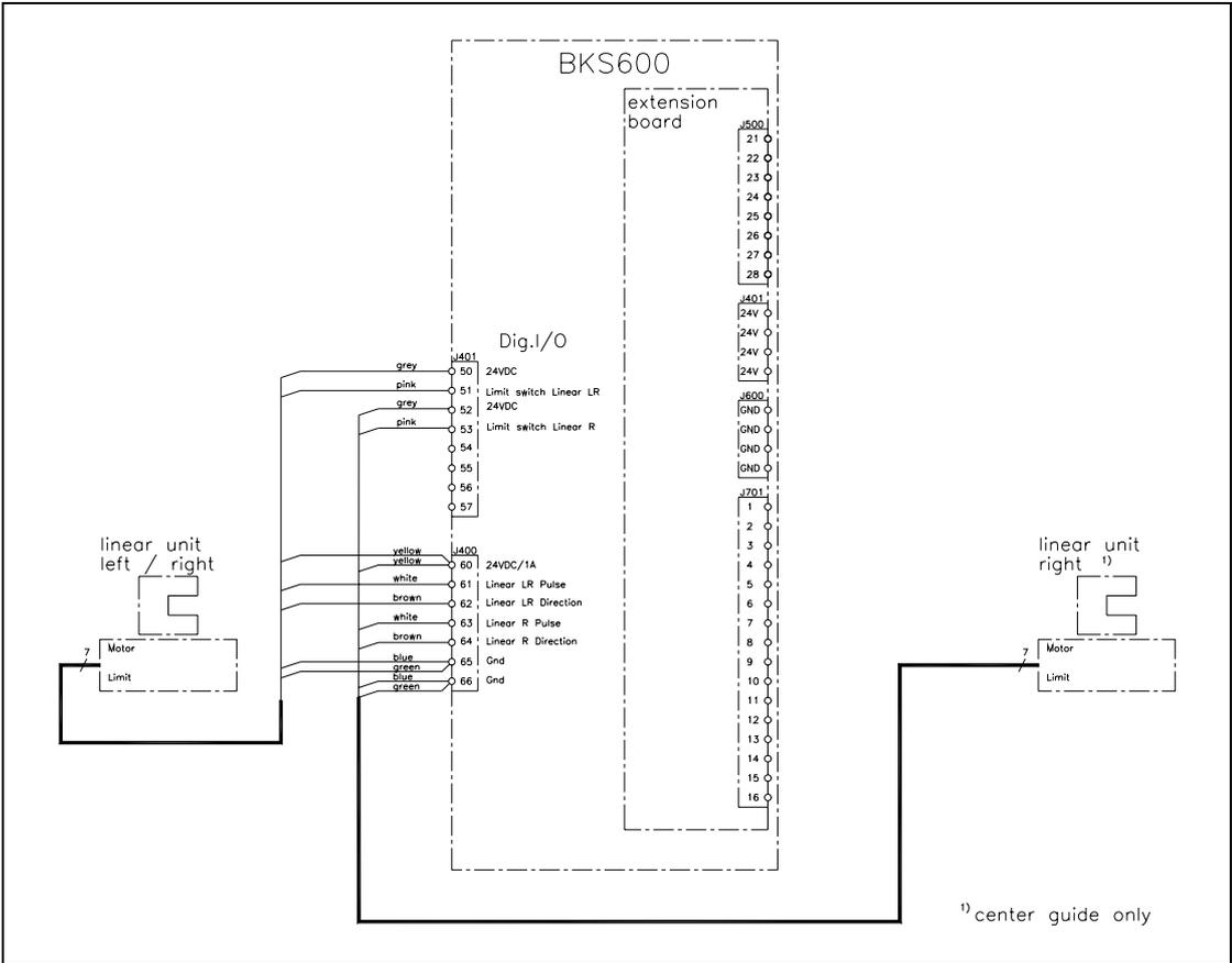
fig. 10: Wiring of the linear units
