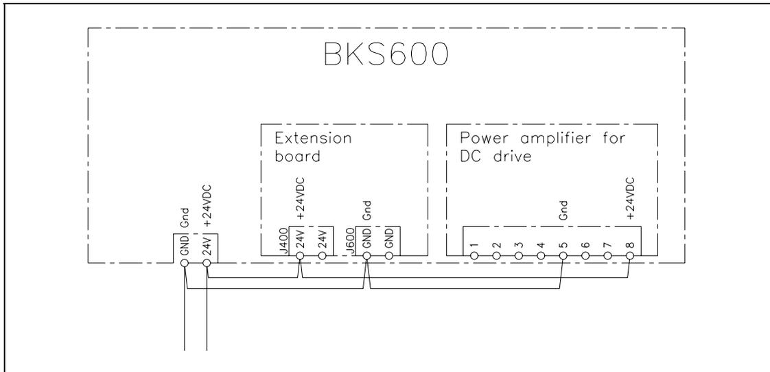
fig. 7: Wiring of the power supply to the electronic unit
