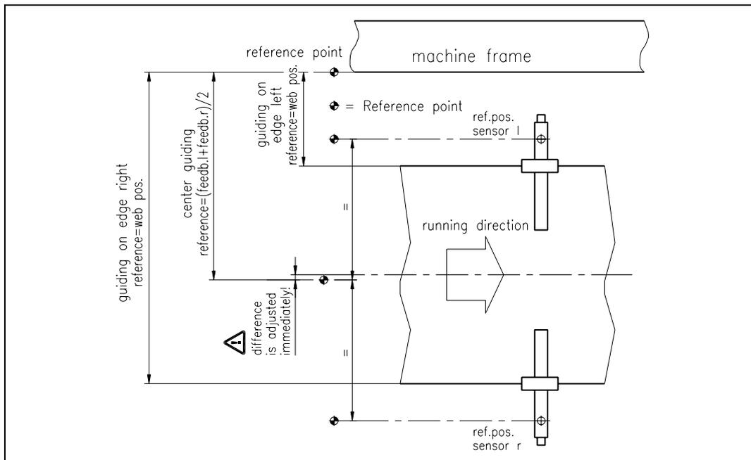
**fig. 20: Calculation of the reference value during automatic start by using linear units (with reference point on the machine frame)**
