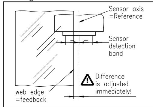
**fig. 18: Calculation of reference position during automatic start** K100005e
