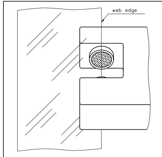
**fig. 17: Aligning of the sensor axis to the web edge** K100004e
