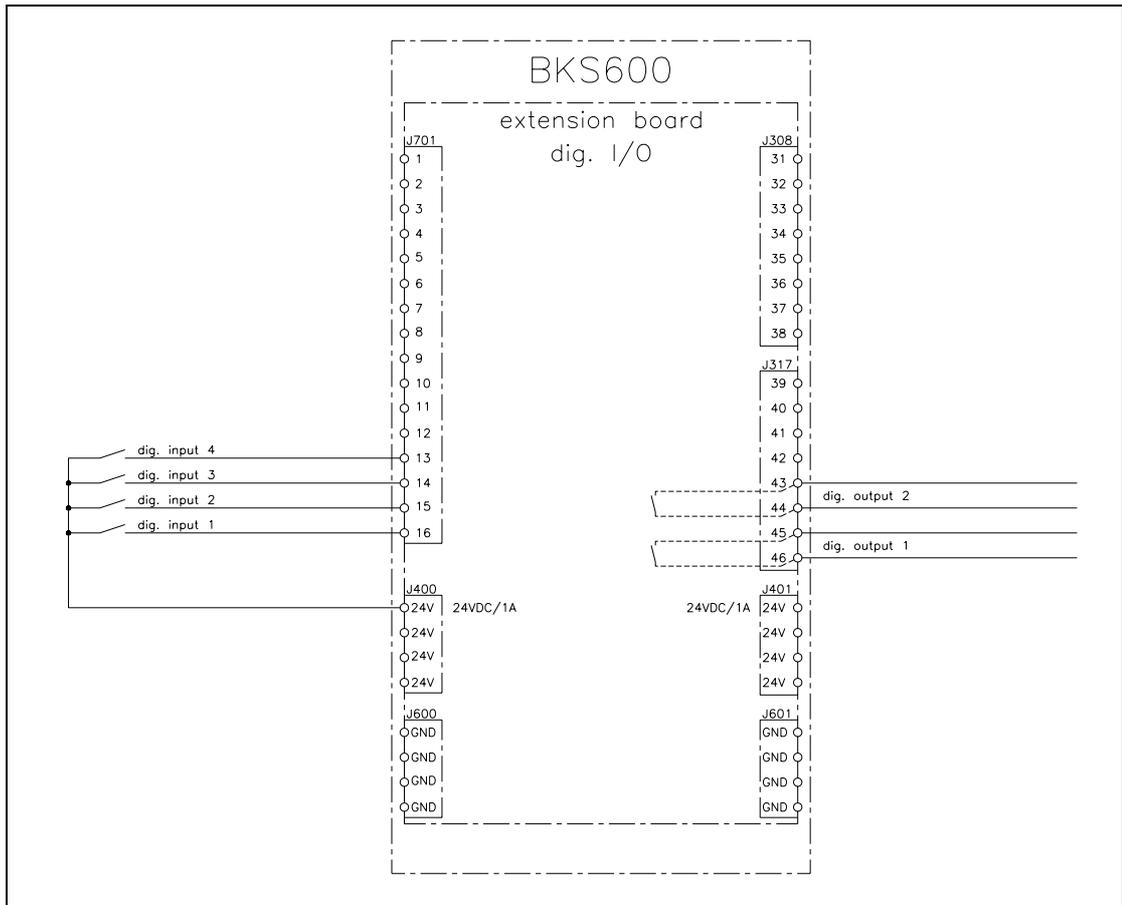
fig. 11: Wiring of the digital inputs and outputs
