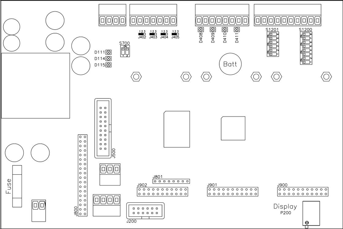
fig. 5: Screw terminal arrangement on the processor board K600028e
