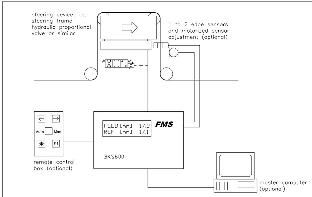
fig. 1: Basic structure of the BKS600A web guide
