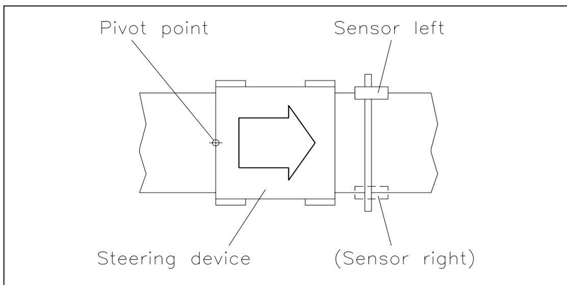
fig. 13: Notice the running direction of the web when mounting the steering device.
