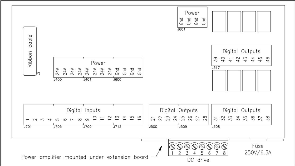
fig. 6: Screw terminal arrangement on the extension board and the power amplifier for the DC drive K600007e
