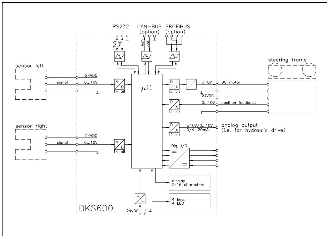
fig. 2: Block diagram BKS600A
