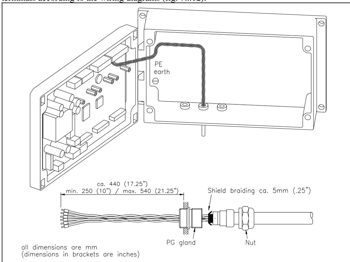
fig. 4: Wiring path inside the housing
