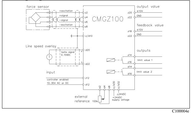
The force sensors are connected using 2x2x0.75mm<sup>2</sup> [AWG 18] shielded twisted pair cable. (With cable length below 15m, 2x2x0.25mm<sup>2</sup> [AWG 23] is also suitable.)
