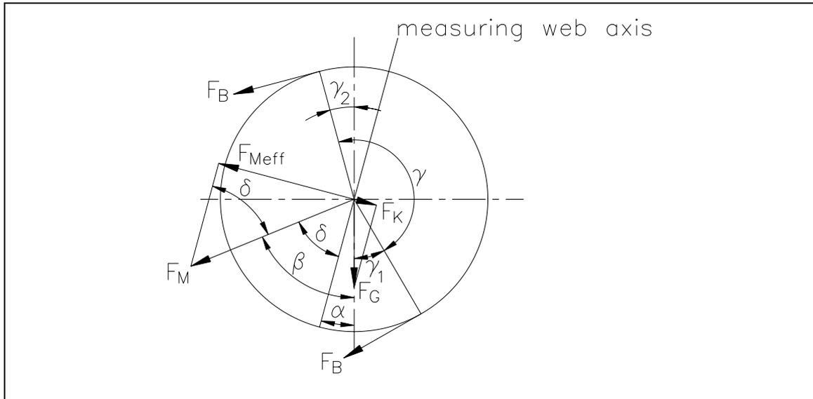
**fig. 14: Force vectors in the FMS force measuring bearing**
