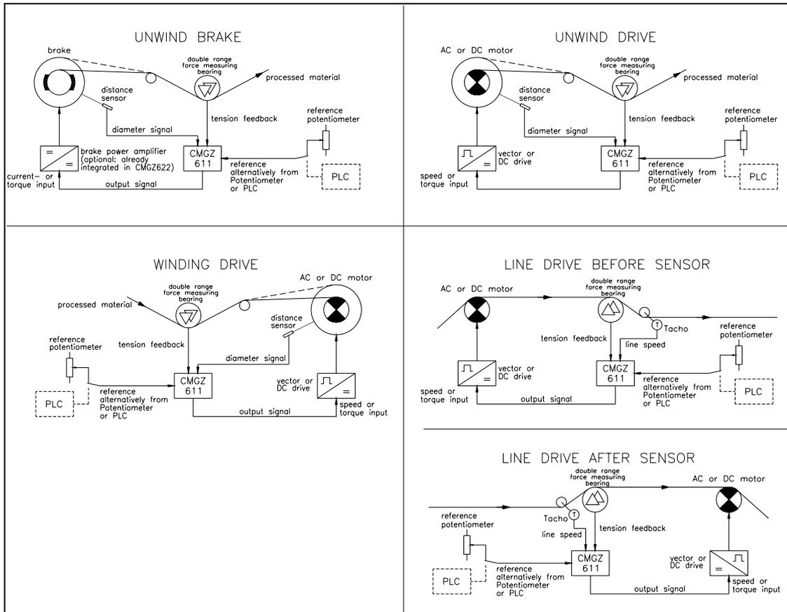
fig. 1: Basic structures of the CMGZ622 configurations
