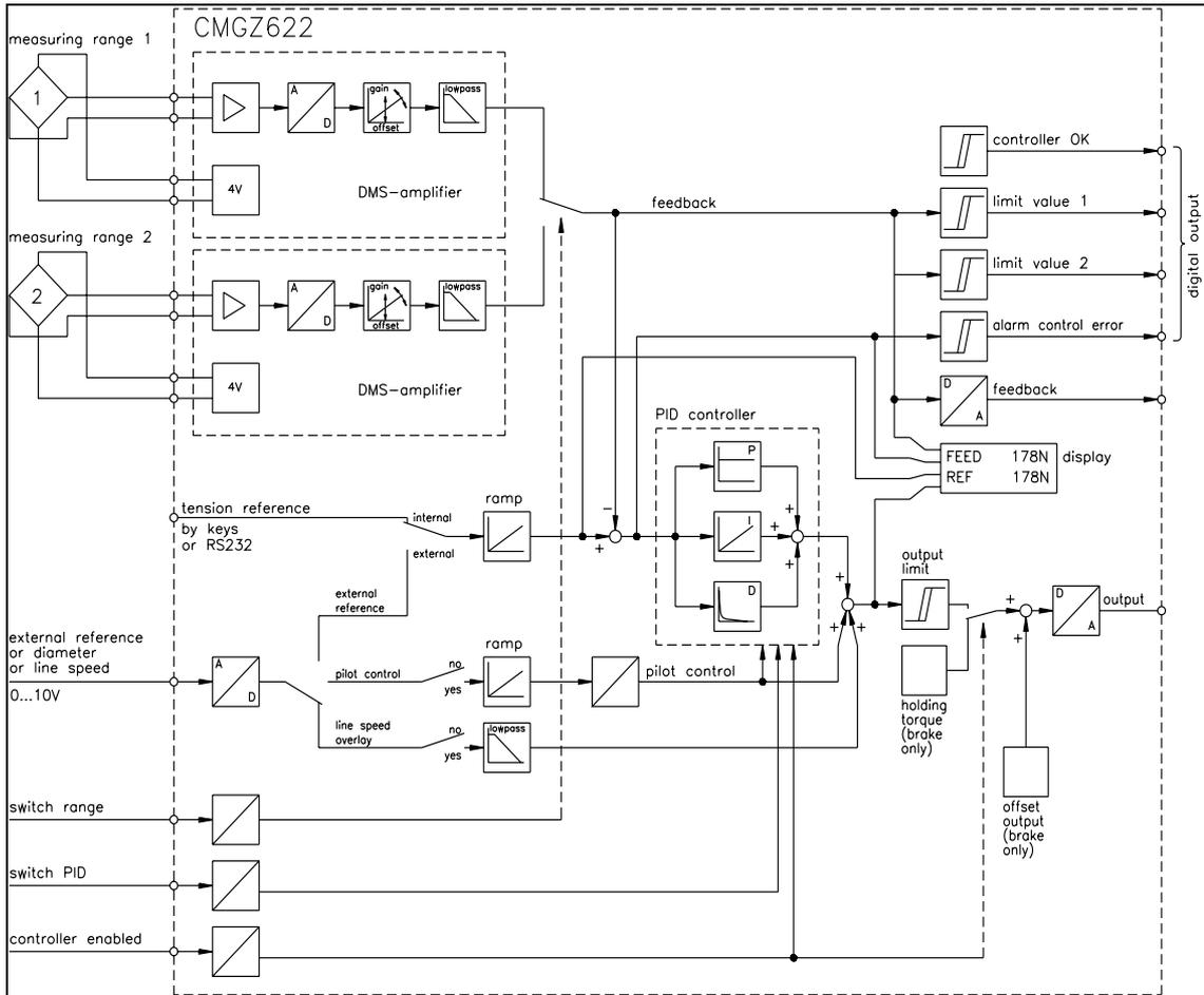
fig. 2: Block diagram of the electronic unit CMGZ622
