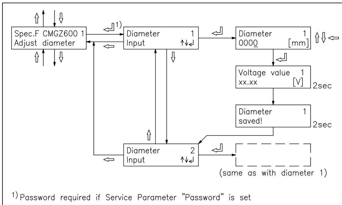
fig. 16: Program flow for special function „Adjust diameter“
