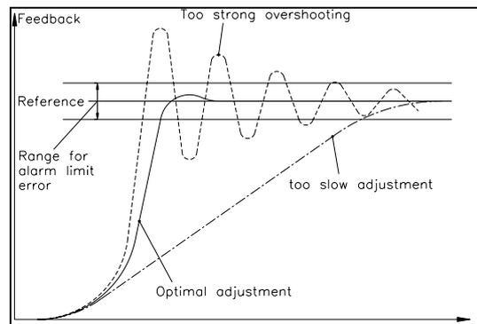
fig. 15: Transient effect of the control system C431013e
