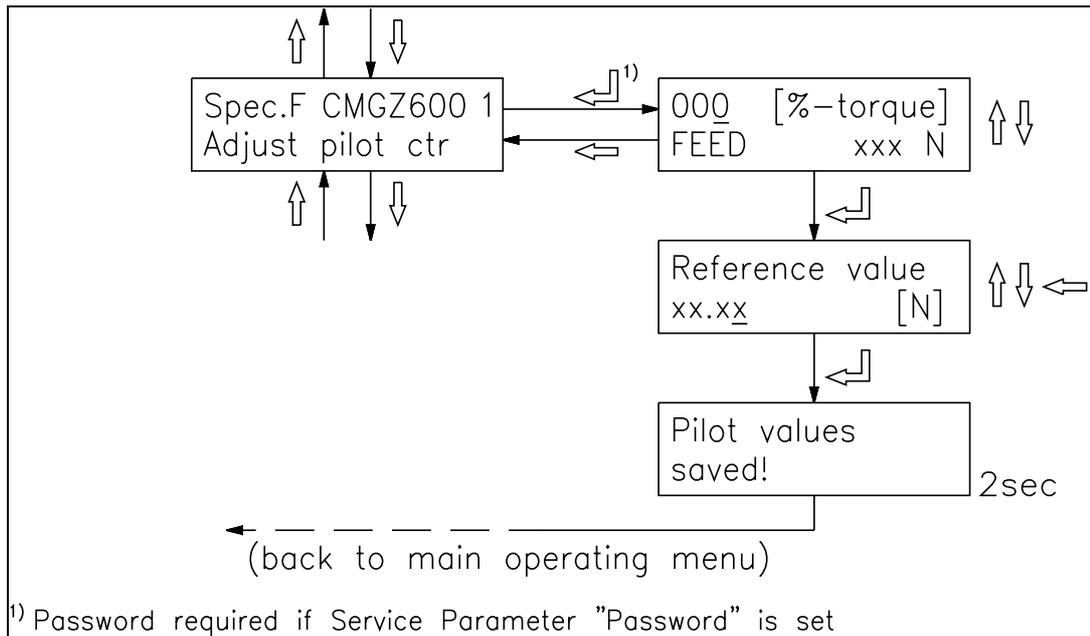
**fig. 17: Program flow for special function „Adjust pilot control“** C611008e
