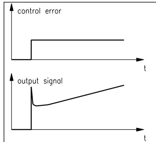
fig 3: Step response of a PID controller C432003e
