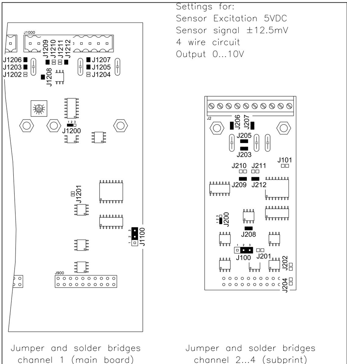
**fig. 23: The jumpers and solder bridges show the settings for processing an FMS force sensor signal.** E600005e
