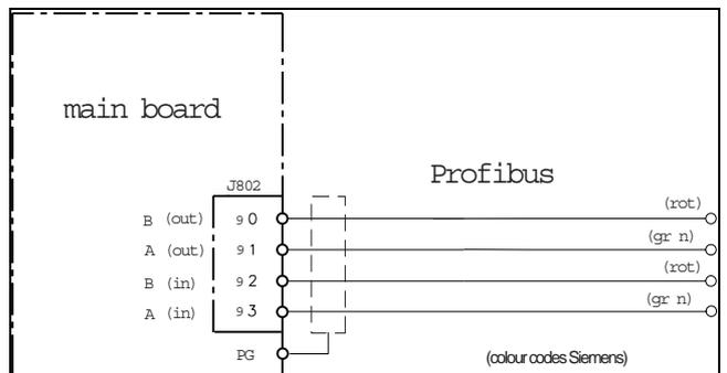
fig. 23A connection Profibus B600030e
