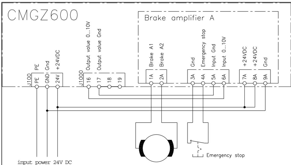
fig. 9: Wiring diagram for integrated brake amplifier CMGZ.B
