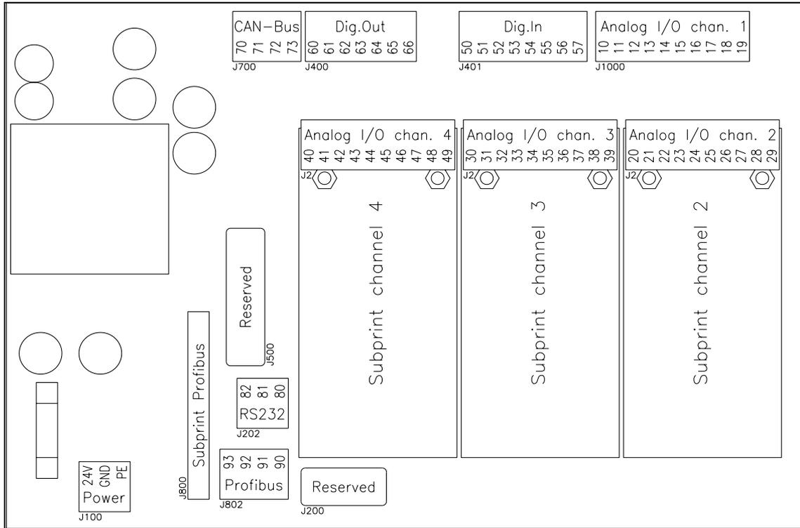
fig. 6: Screw terminal arrangement on the electronic unit
