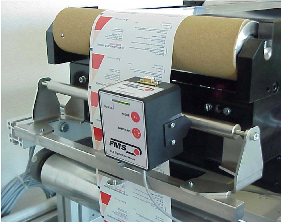
Fig.3: Focus pointer and web stabilization bar
