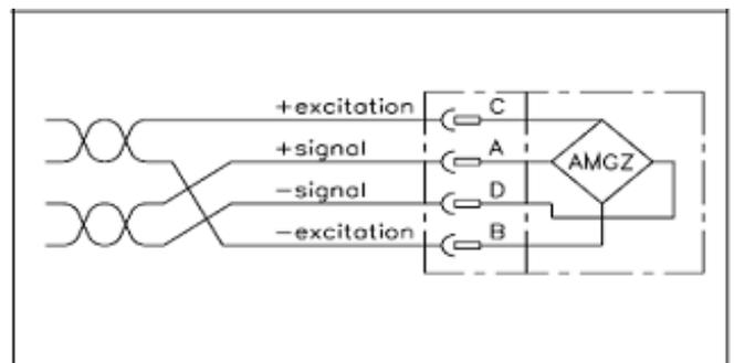
Fig.3: Wiring Diagram
