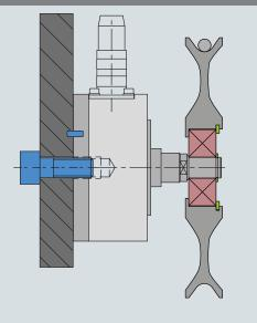
FL - Flat mount with dowel pin for centering
