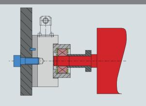
FL - Flat mount with dowel pin for centering
