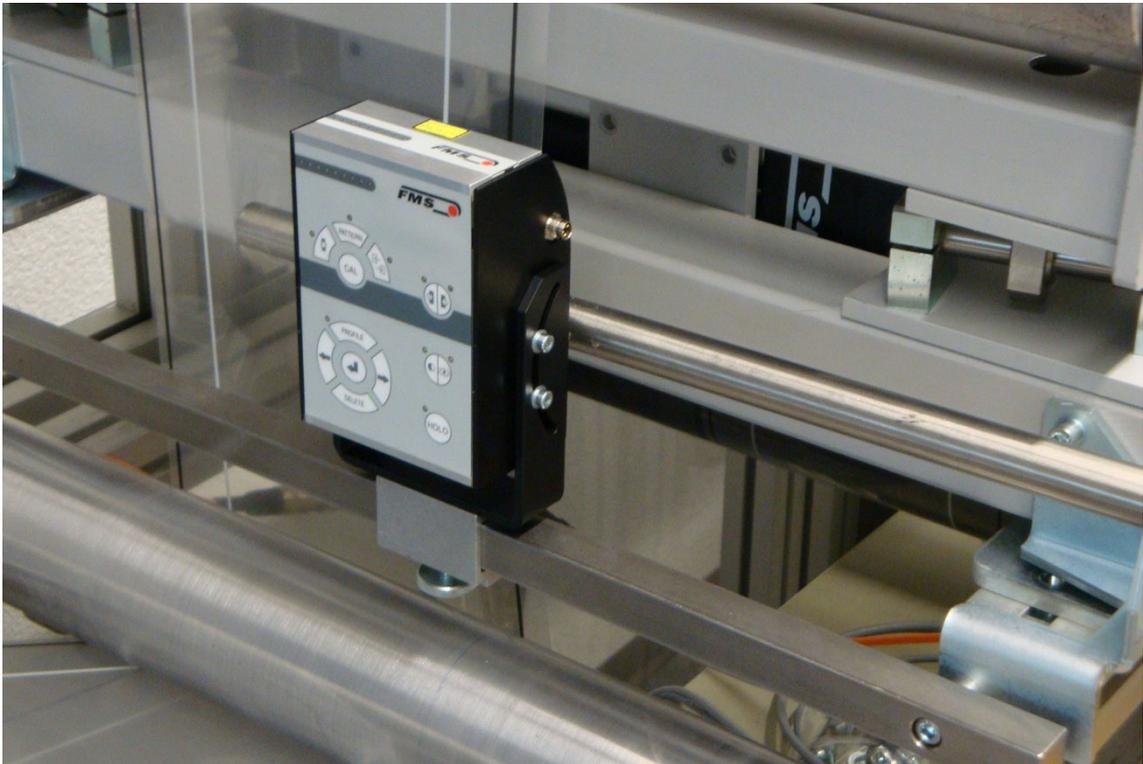
**Fig. 2:** Mounting of sensor on the square bar, view of tilting device DLS200005
