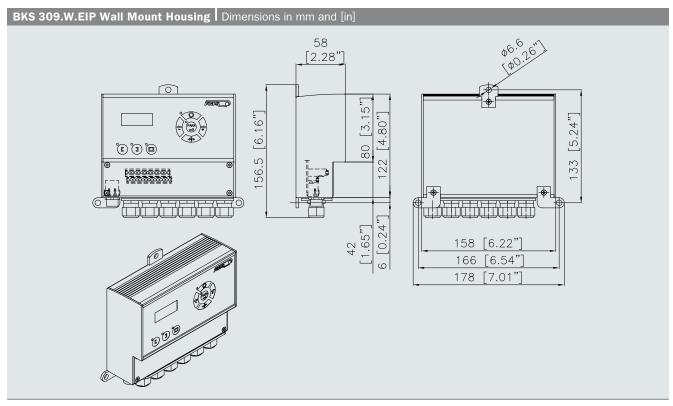
With PG-Gland cable connector; Ethernet: M12 4-Pol D-coded connector (IP65).
