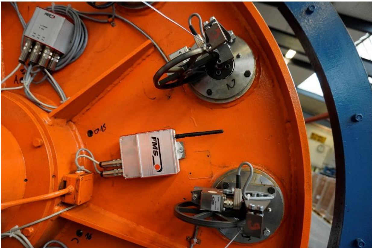
Illustration 3: Lay plate with force sensors, amplifiers and transmitter
