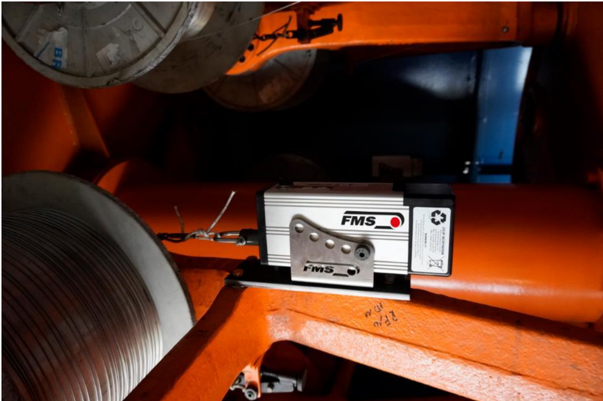
Illustration 4: Single brake actuator for friction brake on cradle
